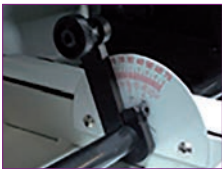
Quick and accurate adjustment of the height by means of an adjustment lever with scale
