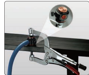
Ground Hog™ Rated at 450 AMPS @ 60% duty cycle (with 2/0 cable)
